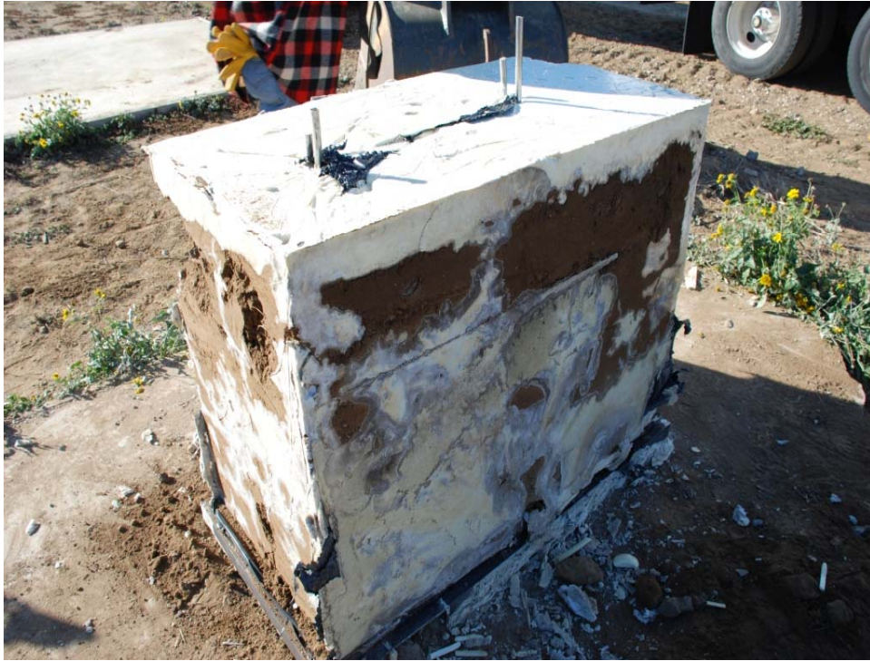
Stabilized soil mass was free-standing after box removed
