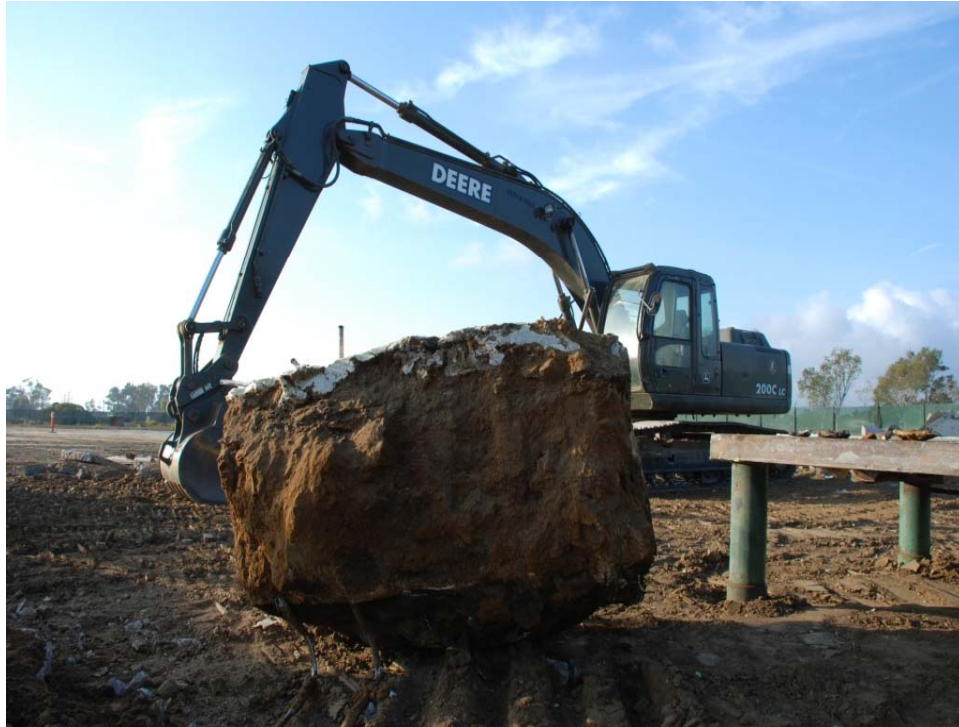
The area of injection was removed intact after the forensic exam
